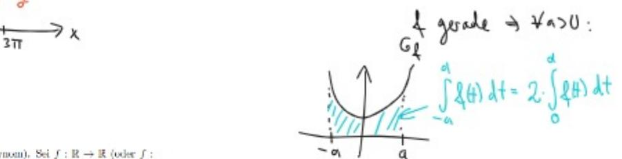
$$\text{Falls } f \text{ gerade } \Rightarrow \forall k \in \mathbb{N}: b_k = 0 \quad \wedge \quad a_k = \frac{2}{T} \int_{-\frac{T}{2}}^{\frac{T}{2}} f(t) \cos(k\omega t) dt = \frac{4}{T} \cdot \int_0^{\frac{T}{2}} f(t) \cos(k\omega t) dt$$
